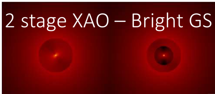
Figure 13: Comparison of an AO-corrected coronagraphic image with the current SPHERE AO design (left) to the proposed additional 2nd faster correction stage (right). Typically 10 times deeper raw contrast is obtained at short separation, up to a radius depending on the 2nd DM number of actuators ( 24 \times 24 in this example).
